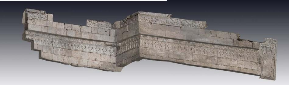
Since even shade was required during the scanning to provide the sensors with a working range, texture colour could not be kept at an even level (see picture above this one). Thus all the texture information that was recorded along with the 3D coordinates was removed and photographic images taken at more favourable light conditions were used for projection of the final texture on to the model (see left and below).
